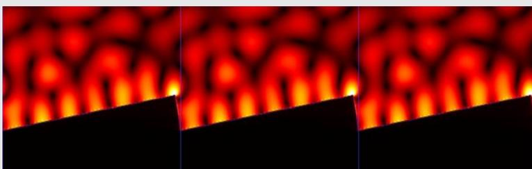
E field reflected by a diffraction grating modelled with RCWA
