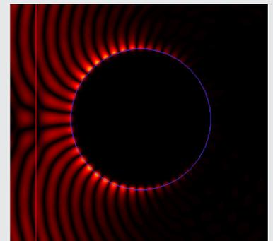
*Mie scattering around gold sphere: field (high frequencies) and finite-element mesh*
