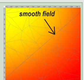
FETD: section of the 3D mesh and  $E_z$  at interface
