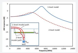
1- and 2-level carrier models: (left) AM response vs frequency for each model (below) epitaxial and quantum well structure
