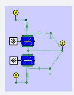
High speed directly-modulated laser/ SOA design. By adding electrical connections to co-modulate the SOA, substantial improvements in the device performance can be obtained.
