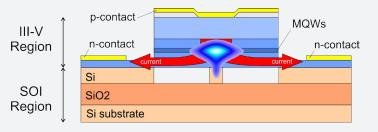
A hybrid silicon III-V laser with current spreading
