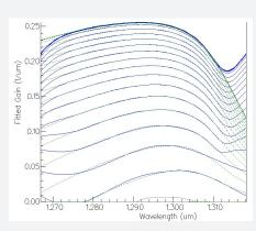
(above) Gain curves computed by Harold for a 3 QW InGaAsP epistructure are shown in green for different carrier densities. PICWave's fitted models are shown in blue. PICWave will import and fit almost all of Harold's other results, including spontaneous recombination, diffusion, refractive index data...
